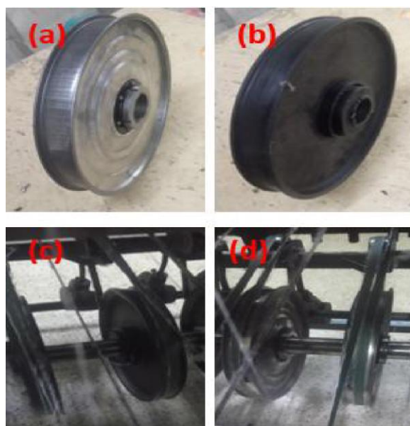
Fig. 3. Metallic T-in cylinder (a), plastic T-in cylinder (b), plastic T-in cylinder mounted in a ring frame (c), and metallic T-in cylinder mounted in a ring frame (d).
