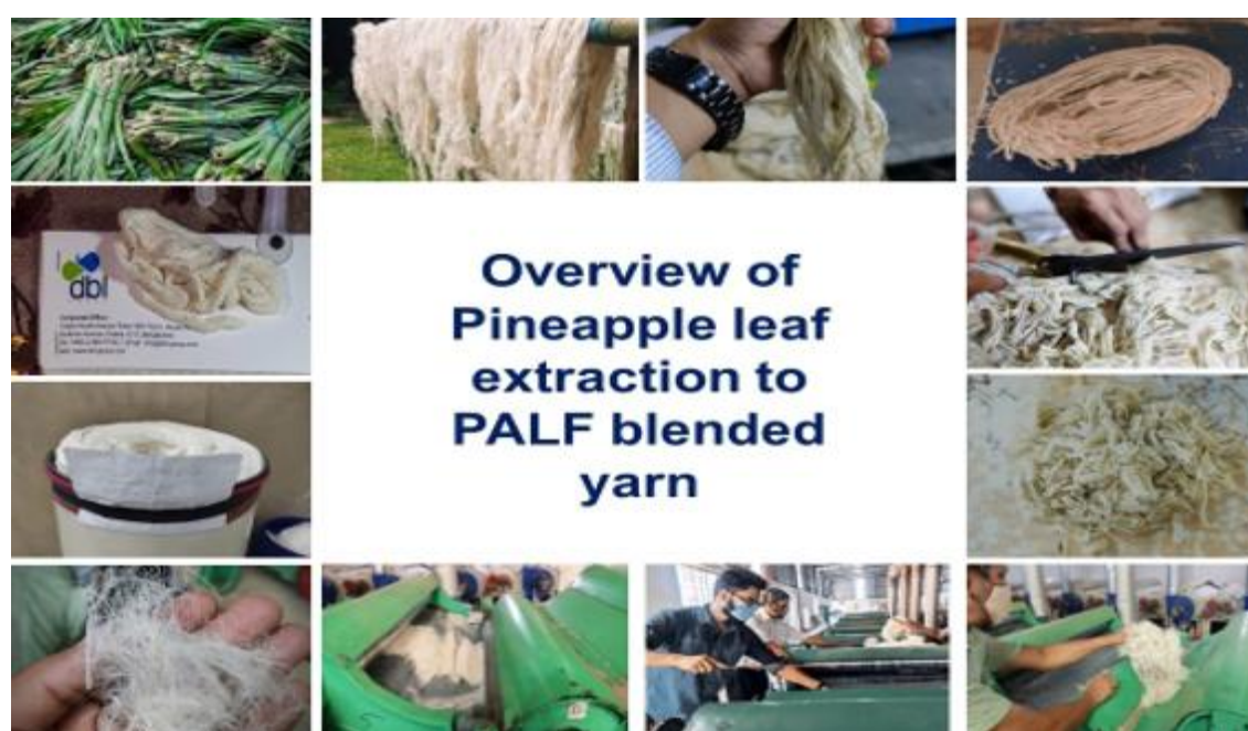
Figure 1. Overview of the process from pineapple leaf fiber (PALF) extraction to blended yarn production. The images depict successive stages including collection of pineapple leaves, fiber extraction, washing, drying, cutting, and blending with cotton and polyester fibers, followed by spinning and preparation of final yarn samples
