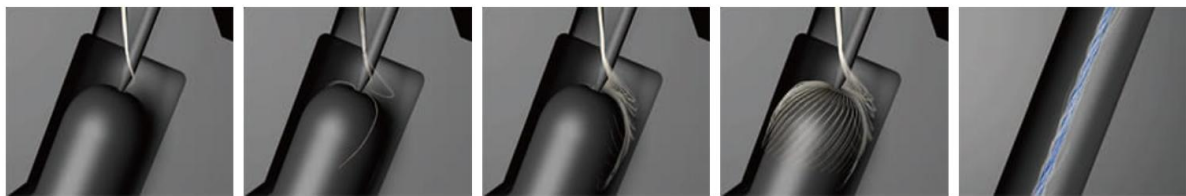
Figure 1: Schematic illustration of the yarn formation mechanism within the vortex spinning chamber, demonstrating how the high-velocity rotational airflow twists the fiber strand [2].
