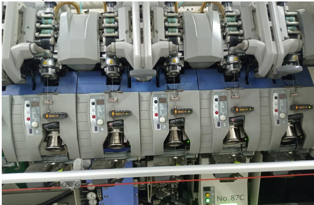
Figure 2: Yarn formation zone of vortex spinning (MVS)
